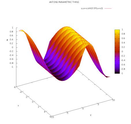
Figure 1: a parametric mode "splot" with hidden3d option (depth sorting) disabled
